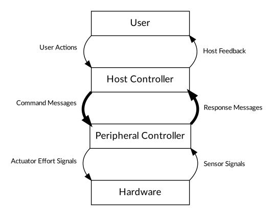
Fig. 3.1: : Simplified functional block diagram showing the interfaces and interactions between the user, the host controller, the peripheral controller, and the hardware. The host-peripheral protocol described on this page specifies the interfaces represented by the diagram's thick edges between the host controller and the peripheral controller.
